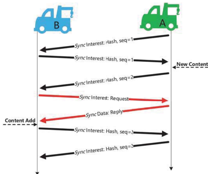
Fig. 3. Synchronization between two nodes
